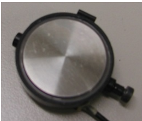
figure 5 Prototype transducer for ultrasound therapy (1 MHz) and frequency response measured in air and water
