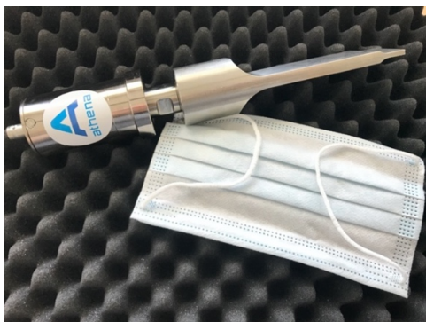
figure 2: Personal protection equipment like breathing masks manufactured by ultrasonic welding
