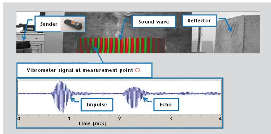
Fig. 5: Refracto-vibrometric measurement of the propagating sound pressure packet of an instrument measuring pulse-echo distance.
