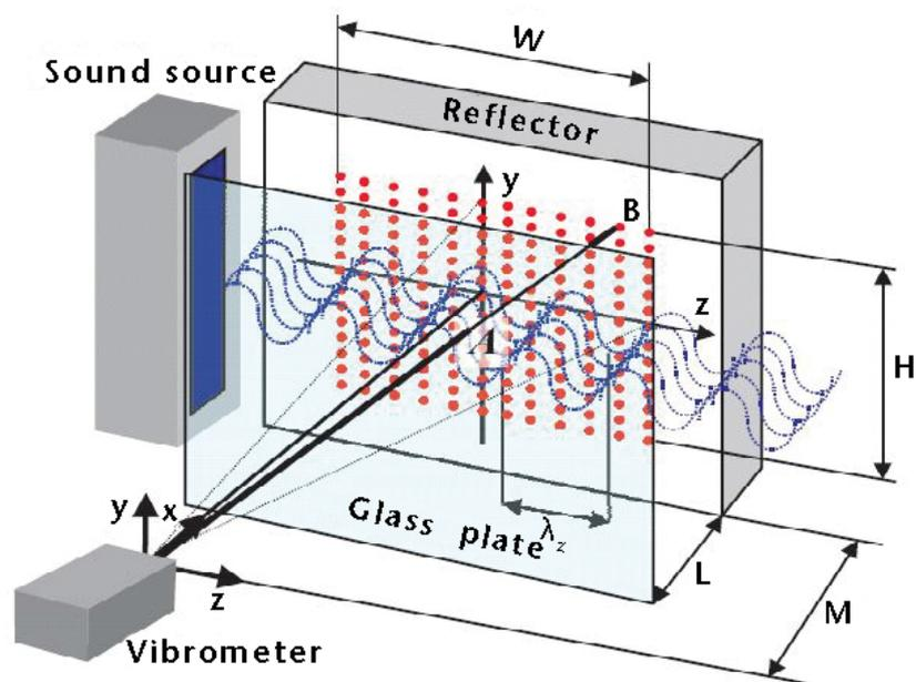
Fig. 2: The arrangement of a Scanning Laser Vibrometer and corresponding reflector to provide Refracto-vibrometry measurements on a propagating sound or ultrasonic plane wave in air (according to Zipser et al. [9]).
