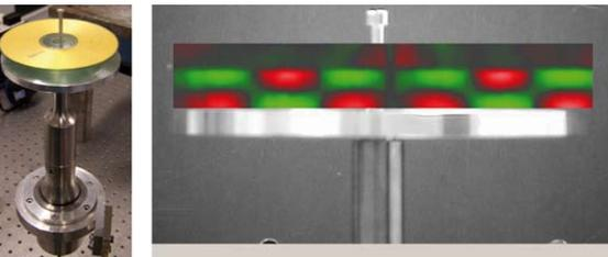
Fig. 4: Ultrasonic vibration of a circular bending plate causes a compact disc to levitate [11]. By means of refracto-vibrometry, an impression of the sound pressure distribution in the resonance sound field can be easily obtained.
