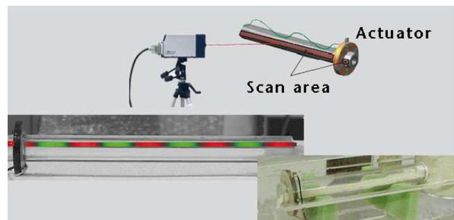
Fig. 1: Scanning laser measurements of an ultrasonic powder metering system showing a deflection shape.
