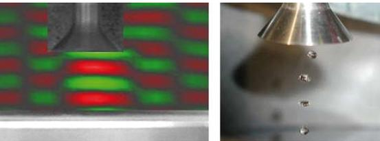
Fig. 3: Sound pressure distribution under an ultrasonic transducer that generates a standing wave in the air (effectively a standing wave positioner according to Lierke [10]). The image on the right shows water droplets which are kept suspended by the standing wave in the sound pressure nodes. The measurements were made jointly with colleagues from the Mechatronics and Dynamics group at the University of Paderborn.
